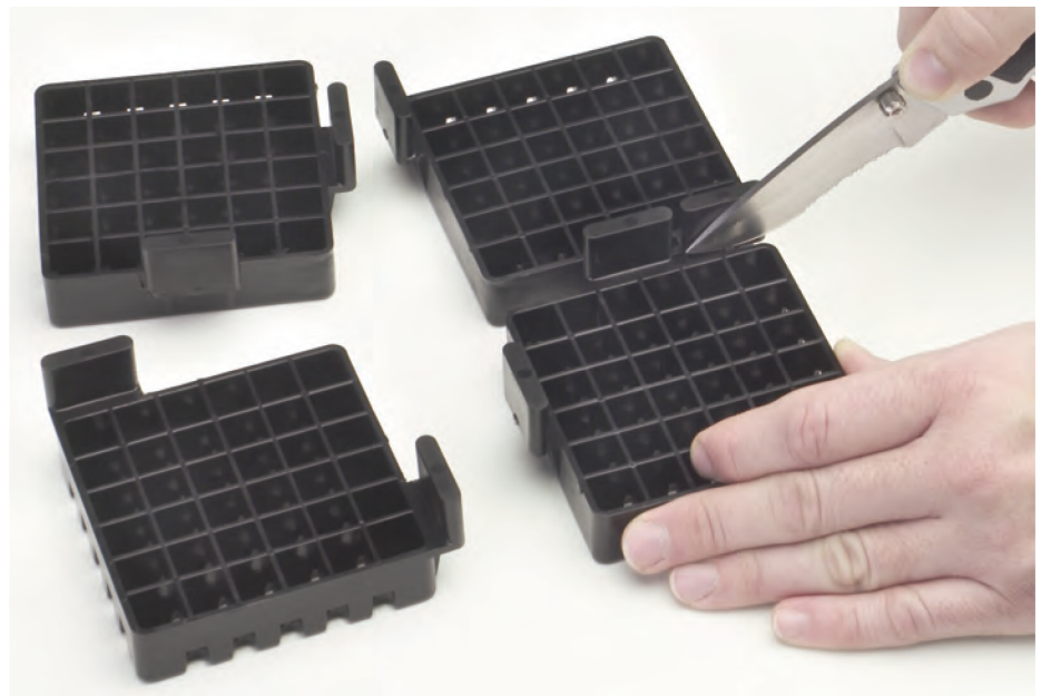
PAVE-EL pedestals and leveling plates (shims) are easily divided into halves and quarters by cutting units at polyethylene bridge points.
